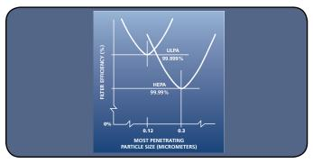
**ULPA filters have an efficiency** of **99.99%** vs 99.99% of HEPA filters, therefore ULPA filters meet HEPA filter efficiency requirement, but at higher efficiency, giving you better operator and product protection.
